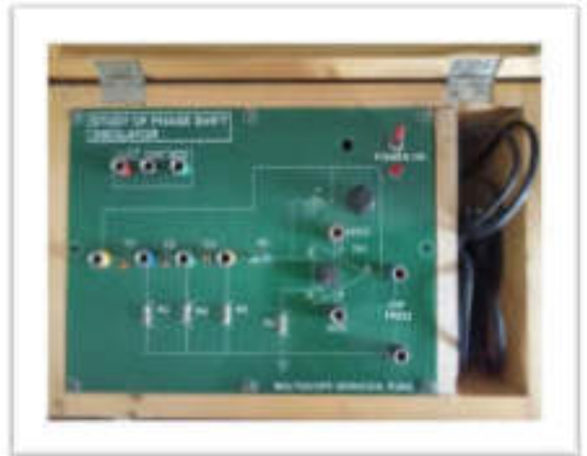
Study of Phase Shift oscillator
